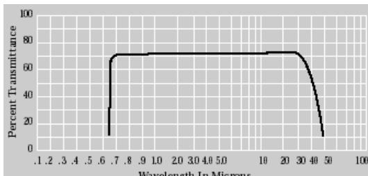
Slightly soluble in water. Not hygroscopic. Soft, hence easily deformed.
