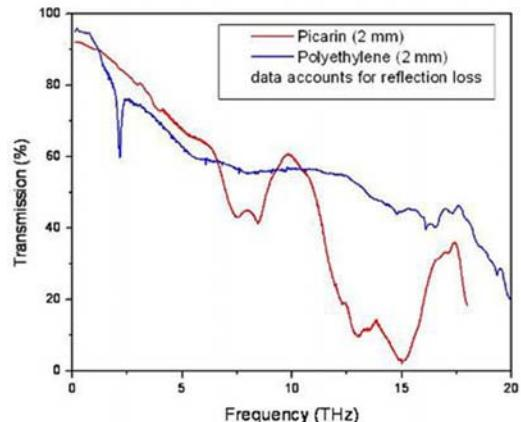
For TerraHz Spectroscopy Applications.
